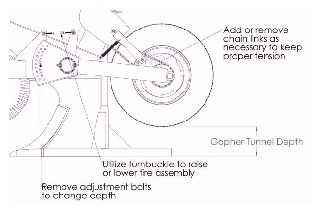
After adjustment reinstall adjustment bolts and torque to 50 ft-lbs.
