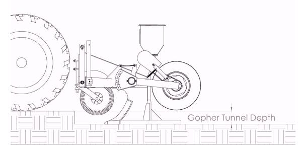
Use a flat level platform to raise the entire tractor the same height as the gopher tunnel. This allows for the machine to be lowered, simulating operation in the field, and adjusted for level.
